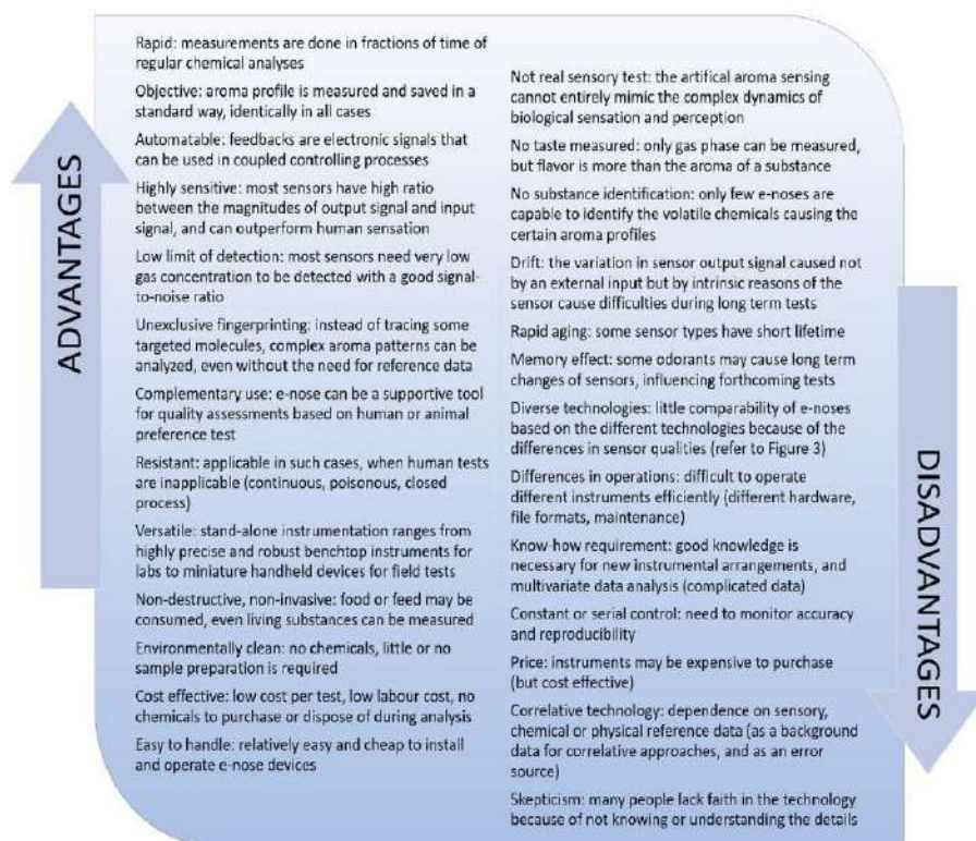
Figure 2. Advantages and disadvantages of electronic nose technologies.
