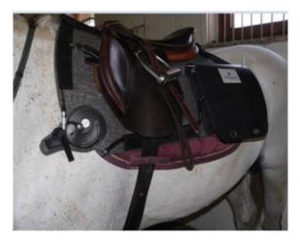
Figure 3a: Overground endoscopy saddle pad (Optomed). Endoscopy was performed using a 1 m long, 9.8 mm diameter endoscope attached to a specific saddle pad on the horse, designed to carry the processor and the recorder. (Source: MTA - SZIE Large Animal Clinical Research Group)
